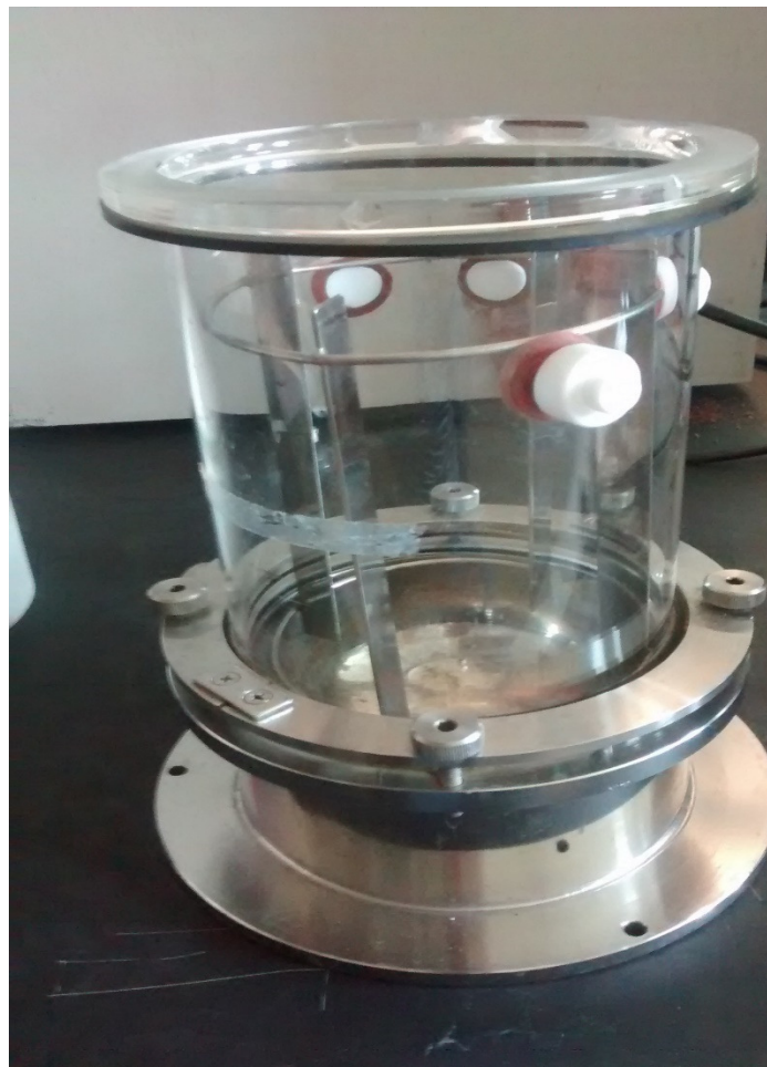
Figure 3.8: Lab-scale vessel. Tape line indicates the target fill level
