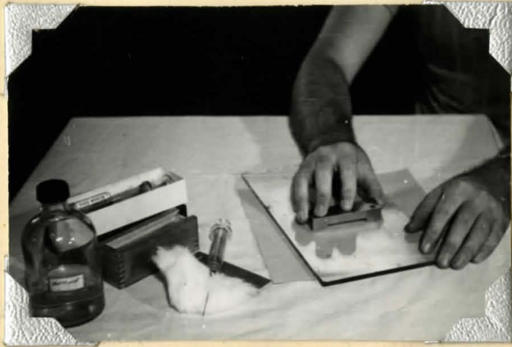
a. Casting of Film ( Bird Applicator)
