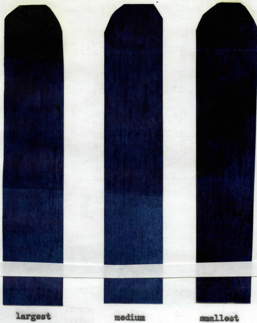
Figure 6. Effect of Particle Size on Bronze in Blown Castor Oil.
