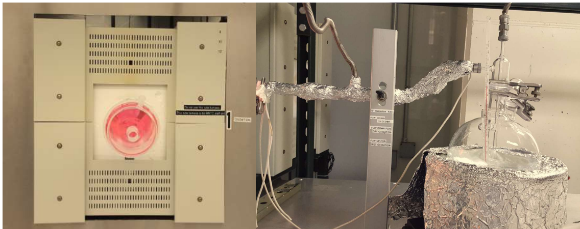
Figure 4.10. (a) Front view of the three-zone tube furnace (b) Quartz bubbler system for the wet oxidation.
