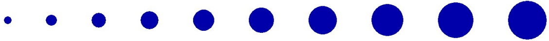
Figure 3.3. Features on the photomask (containing circular features from 200 \mu\text{m} to 1100 \mu\text{m} in diameter).
