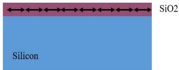
Figure 4.6. Internal compressive stress of the thermal oxide thin film.
