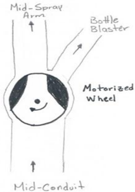
Figure 12: Electric motor operate concept to open/closes the Mid Spray Arm or Bottle Blaster.
