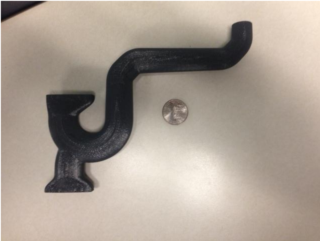
Figure 31: FDM prototype of the Hydraulic Switch with a quarter shown for scale
