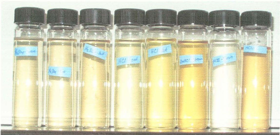
Figure 2-3. The filtrates from the different extraction methods show a wide variation in color. The Mehlich3 extract (second from right) is clear indicating iron is not present. \text{HClO}_4 and 2 M HCl extracts have high concentrations of iron (indicated by intense yellow color).
