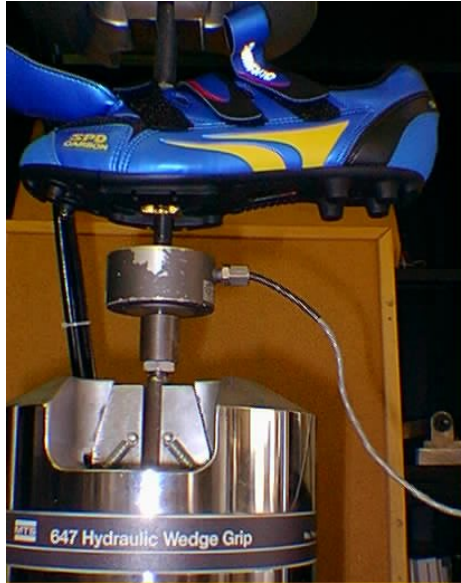
Figure 30. MTS three-point bending arrangement with shoe in place. The fixture was held stationary while the force transducer was thrust upward into the metal cleat.
