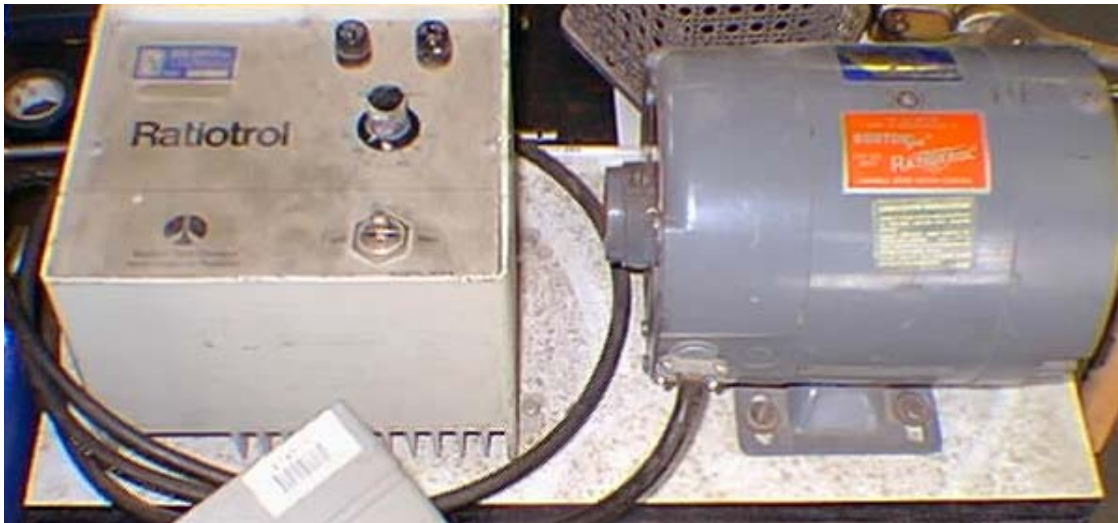
Figure 19. Controller unit and electric motor used to turn the simulated crank mechanism for testing the magnetic resistance unit. The system was adjusted to simulate a 90-RPM crank speed.
