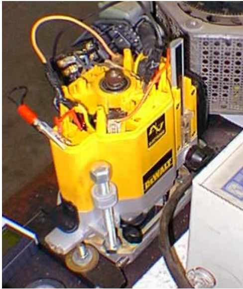
Figure 10. Electronic plunge router used to spin the magnetic resistance unit. The router was chosen because of its ability to reach rotational speeds of up to 22,000 RPM.
