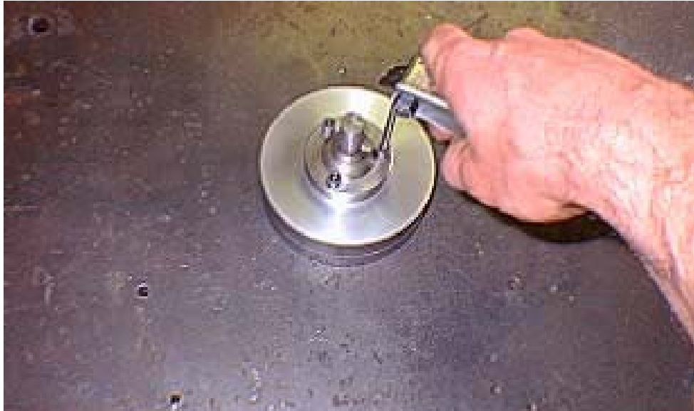
Figure 14. Adapter used to connect the router motor to the magnetic resistance unit.
