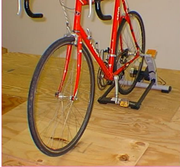
Figure 21. Bicycle and Tacx magnetic resistance unit.
