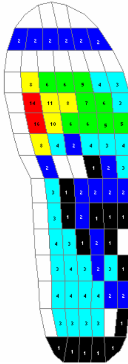
Figure 37. Two-dimensional planar stress plot from Pedar software. The red indicates the highest stress ( \sim 14 \text{ N/cm}^2 ), followed by yellow, then green, then light blue. Dark blue and black indicate very low stress values.
