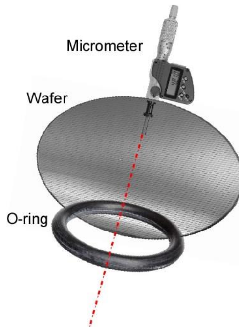
Figure 7.1 Setup for sensitivity study at different stresses.
