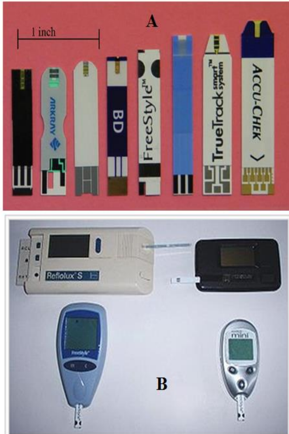
Figure 1.1: A) An assortment of electrochemical miniature blood glucose test strips sampling 1 \mu\text{L} or less from several manufacturers [10]. B) Four generations of portable, battery-powered BGM meters with sampling times of 5 seconds to 2 minutes.
