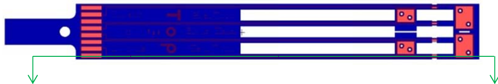
Figure 3.1 (a): PMEA device. Green arrow lines show the approximate location of the cross-sectioning. The device design used for the example is version 3.
