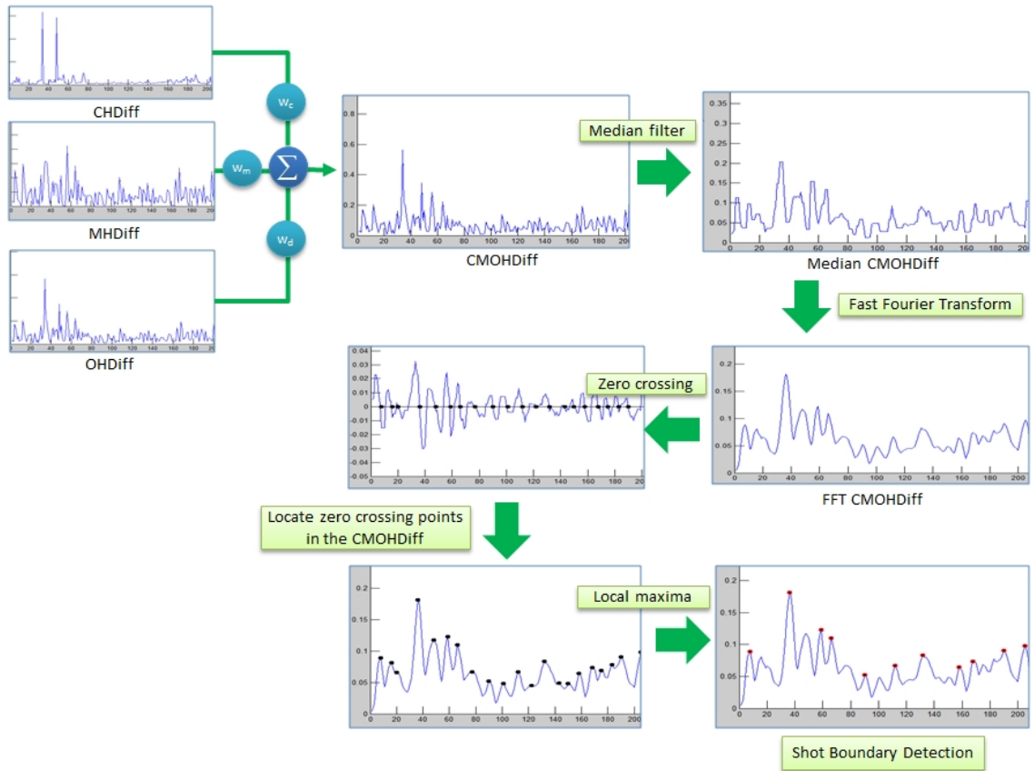
Figure 3.9: Different steps of the proposed SD_FD.
