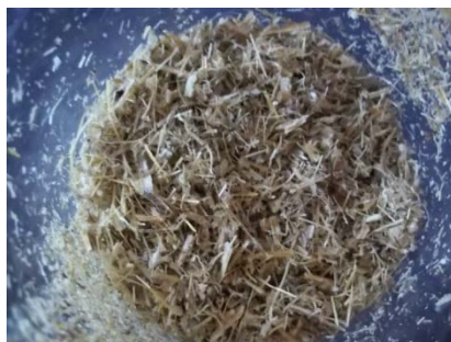
FIGURE 9: Dilute-base pretreated corn stover after washing
