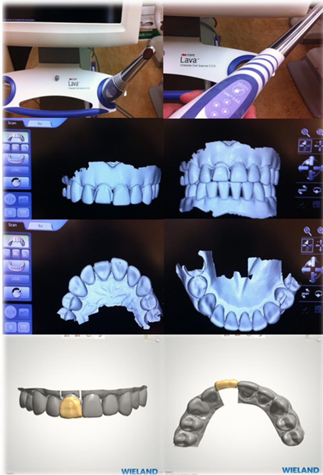
(4) Complete arch digital impressions (Lava COS) of the dentofrom. Impressed veneers were sent for virtual IPS e.max CAD/CAM milling and processing.
