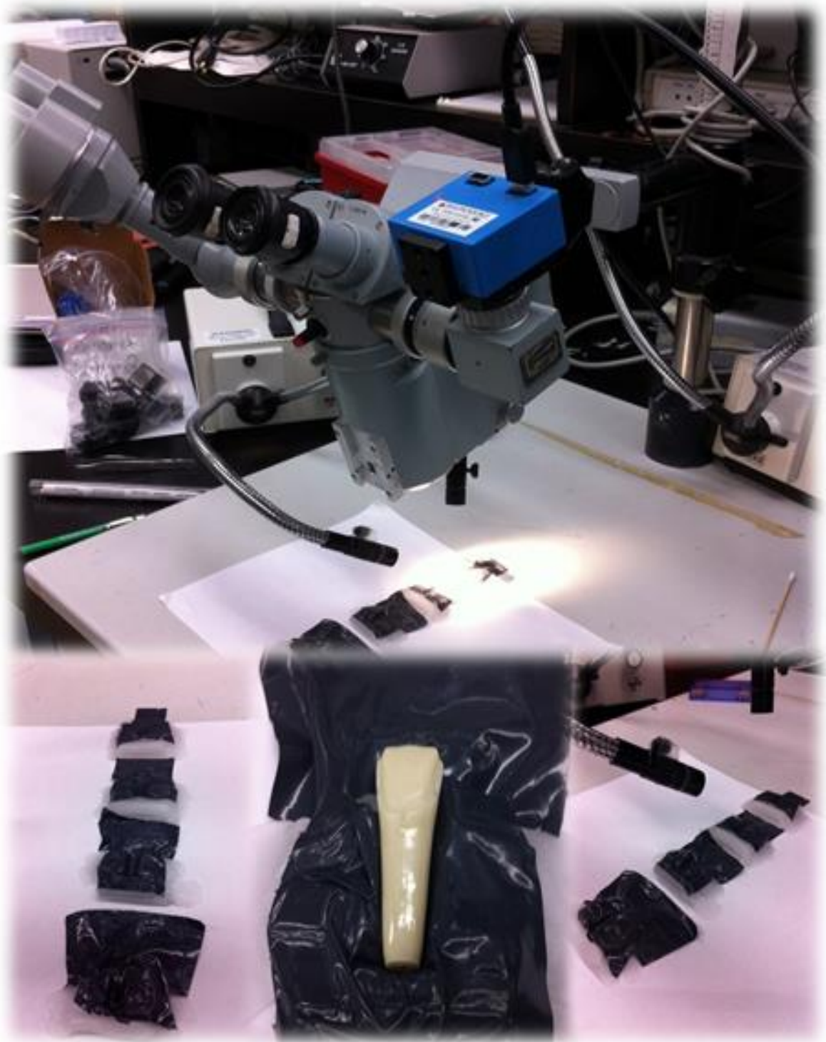
(5) Marginal integrity testing using a stereomicroscope (45X). All veneers were fitted on the cast using wax moldings for normal resting position during imaging.
