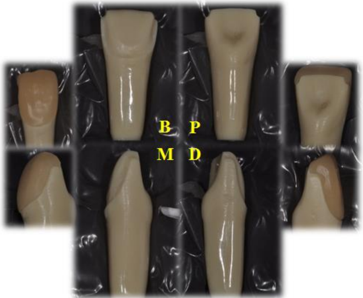
(6) Orientations of fitted veneers in buccal (B), palatal (P), mesial (M), distal (D) position. Specimens were not cemented for any measurement.
