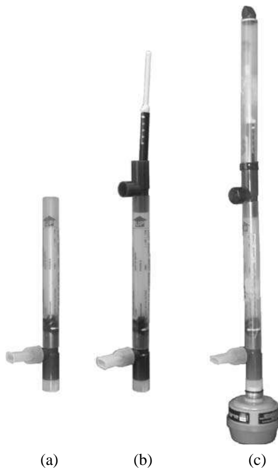
Figure 2. EBC and EBV collection devices: a) The commercially available RTube™; b) The RTube™ was modified for EBV collection by the addition of a plastic fitting to hold a SPME fiber for active sampling; c) The additional modification of the RTube™ to provide an enclosed environment for SPME sampling as well as the addition of a respirator to purify inhaled air (Martin et al. , 2010)
