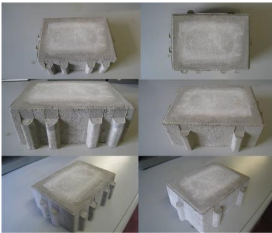
Figure 16. Paver block types (a) Coventry I® (b) Eco-Cobble® (c) Eco-Paver® (Antunes 2013)
