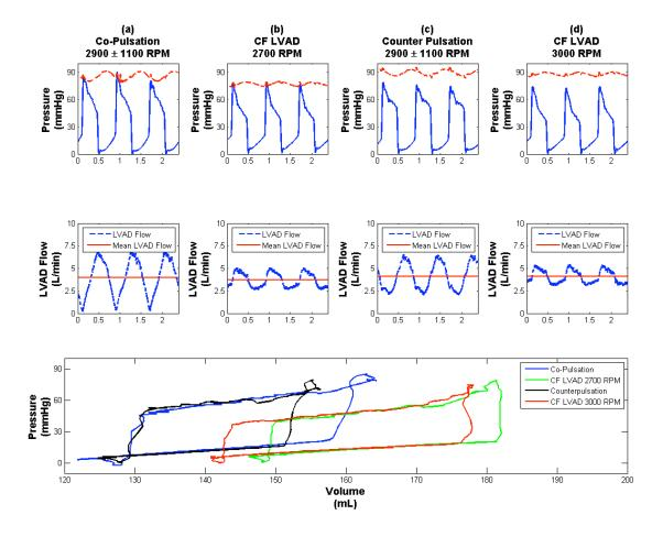
Figure 15: Aortic pressure, left ventricular pressure, LVAD flow, mean LVAD flow and pressure volume loops for (a) co-pulsation LVAD modulation at 2900±1100 RPM, (b) CF LVAD at 2700 RPM, (c) counter pulsation LVAD RPM modulation at 2900±1100 RPM, and (d) CF LVAD at 3000 RPM. Co-pulsation at 2900±1100 RPM and CF LVAD at 2700 RPM had similar mean LVAD flows. Further, counter pulsation at 2900±1100 RPM and CF LVAD at 3000 RPM had similar mean LVAD flows.
