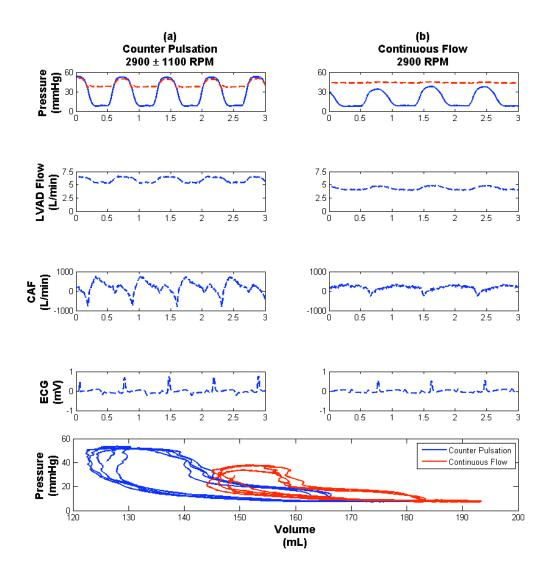
Figure 26: Aortic pressure, left ventricular pressure, LVAD flow, coronary artery flow (CAF), ECG, and pressure volume loops for counter pulsation LVAD RPM modulation (2900 $\pm$ 1100RPM) (mean RPM  $\pm$  modulation RPM) and non-modulated LVAD RPM (2900RPM).
