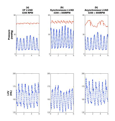
Figure 27: Aortic pressure, left ventricular pressure, left ventricular volume for Normal CF LVAD, Synchronous CF LVAD (3200±800RPM), and asynchronous CF LVAD (3200±800RPM) (mean RPM ± modulation RPM). Synchronous CF LVAD modulation increases AoP Pulsatility while maintaining consistent ranges of left ventricular pressure and volumes. Asynchronous CF LVAD modulation at 19 BPM increases pulse pressure over synchronous modulation while creating varying left ventricular pressure volumes.
