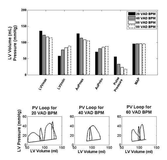
Figure 11: Maximum and minimum values of left ventricular volume (LVV) and aortic pressure (AoP), pulse pressure, mean arterial pressure (MAP), and ventricular pressure-volume loops showing the varying ventricular pressures and volumes for different modulation rates of CF LVAD. Specifically, higher left ventricular volume variability occurs at lower CF LVAD flow modulation rates.
