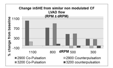
Figure 21: Percent change in SHE during co-pulsation and counter pulsation LVAD RPM modulation from CF LVAD of similar mean flow for base RPMs of 2900 and 3200 for RPM modulation amplitudes of 1100 RPM, 800 RPM, 500 RPM, and 300 RPM.
