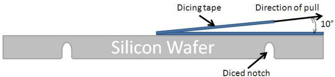
Figure 2-2. Dicing tape removal scheme.
