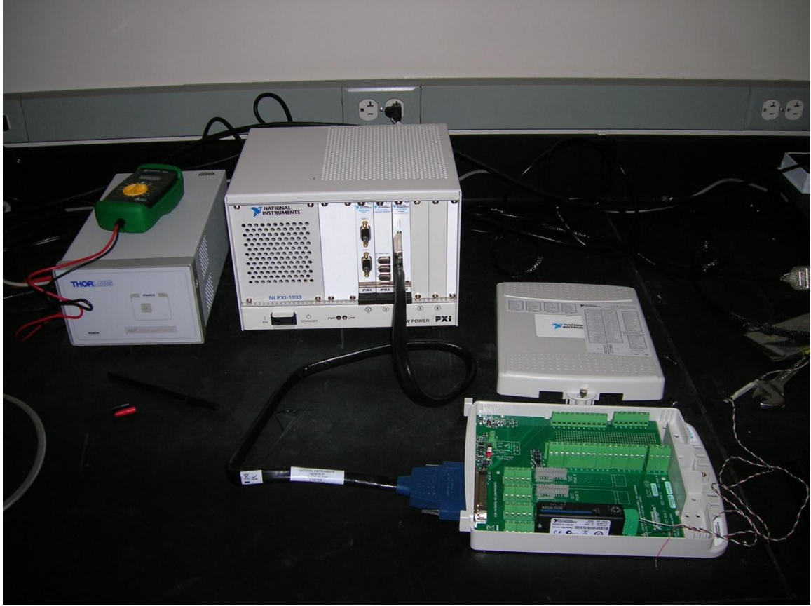
Figure 2-20. Actuator controller, data acquisition system, and amplifier.
