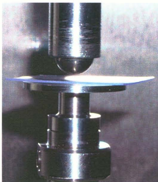
Figure 5. Film indentation using spherical indenter.
