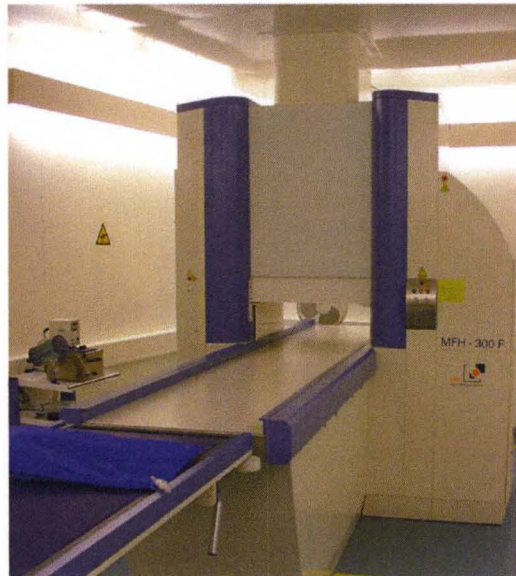
Figure 1.6. AMF applicator for humans: NanoActivator TM , MagForce Nanotechnologies AG, Berlin. A fiber-optic thermometry unit is part of the applicator. Image was taken from Magforce website.
