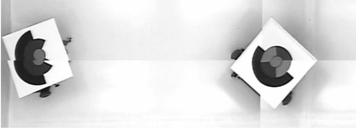
FIGURE 8—A gray-scale image of a section of the testbed with two robots. The cameras were carefully tuned so that they would combine well in the center of the testbed. The robot on the right is in the center and there is a nice image of the pattern. Although the image is nice here, that is not the case for another area of the testbed. The robot on the left shows the schism effect of lens distortion.
