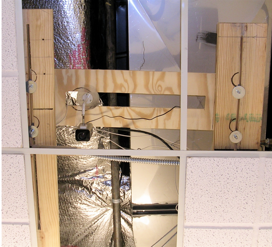
FIGURE 11 – Mounting beams used to support cameras. Slotted holes allow them to be mounted anywhere along the beam for flexibility during calibration.
