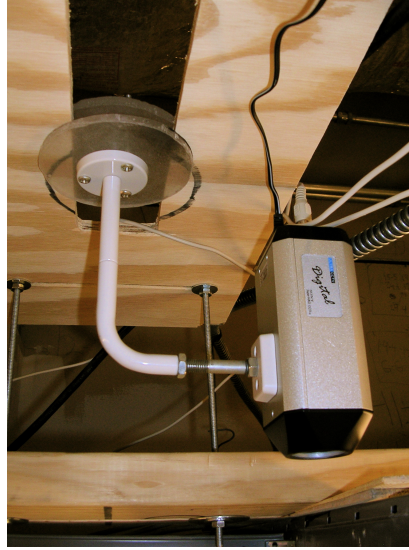
FIGURE 13 – Close-up of mounting brackets or discs used to attach L-arm to mounting platform. The discs sandwich the platform, providing a solid base while still allowing the cameras to rotate, if needed.
