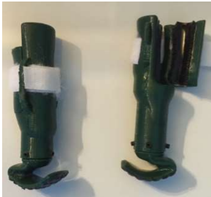
FIGURE 51- Prosthetic Devices After The Acetone Vapor Bath And Modifications.
