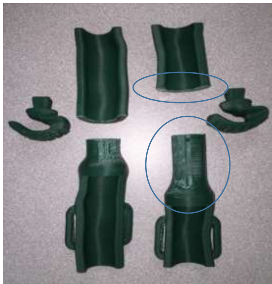
FIGURE 49- Prosthetic Devices After Supports Are Removed, And Surfaces Sanded Down.
