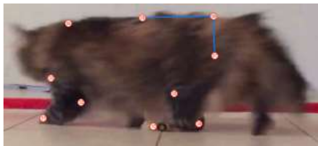
FIGURE 74- Lumbar Spine Angle Gait Data and Reference Image. Grey Shade Indicates Swing Phase.
