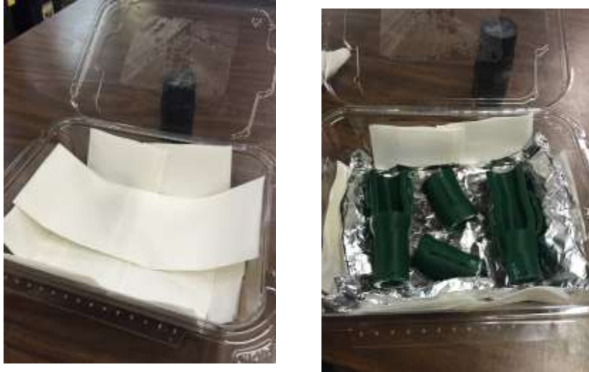
FIGURE 50- Acetone Vapor Bath Setup.
