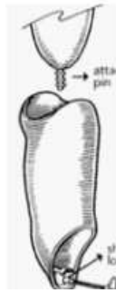
FIGURE 12- Diagram Of Prosthetic Socket Pin Anchoring System.
