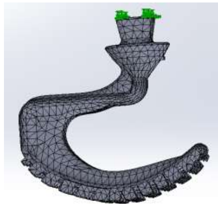
FIGURE 34- Beta Prototype Design Fixed Geometry And Finite Element Mesh In Fatigue Analysis Simulation.
