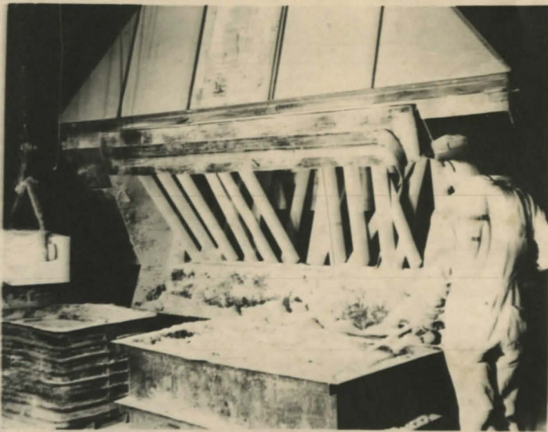
Fig. 11. Can cleaning under canopy hood
