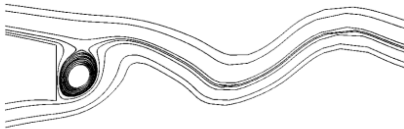
FIGURE 5 - Lower trailing edge vortex formation (van Dam 2009)
