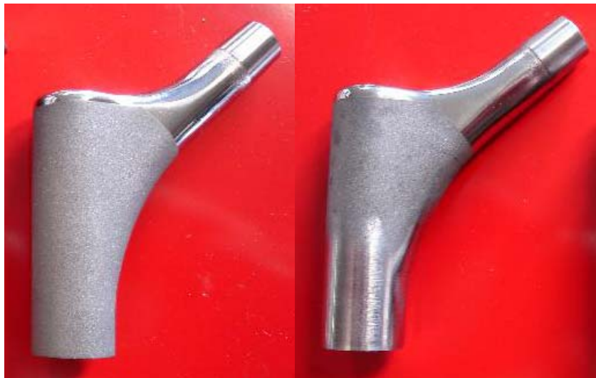
FIGURE 26. Modular body before (left) and after (right) the polishing process.
