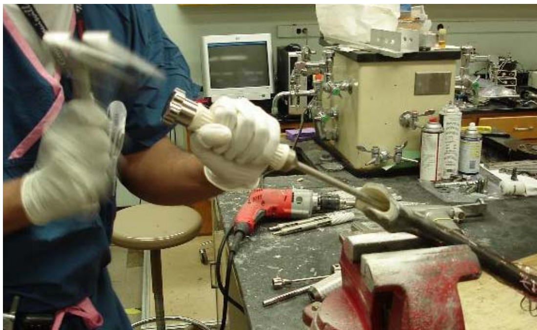
FIGURE 23. Orthopedic surgeon inserting modular stem.
