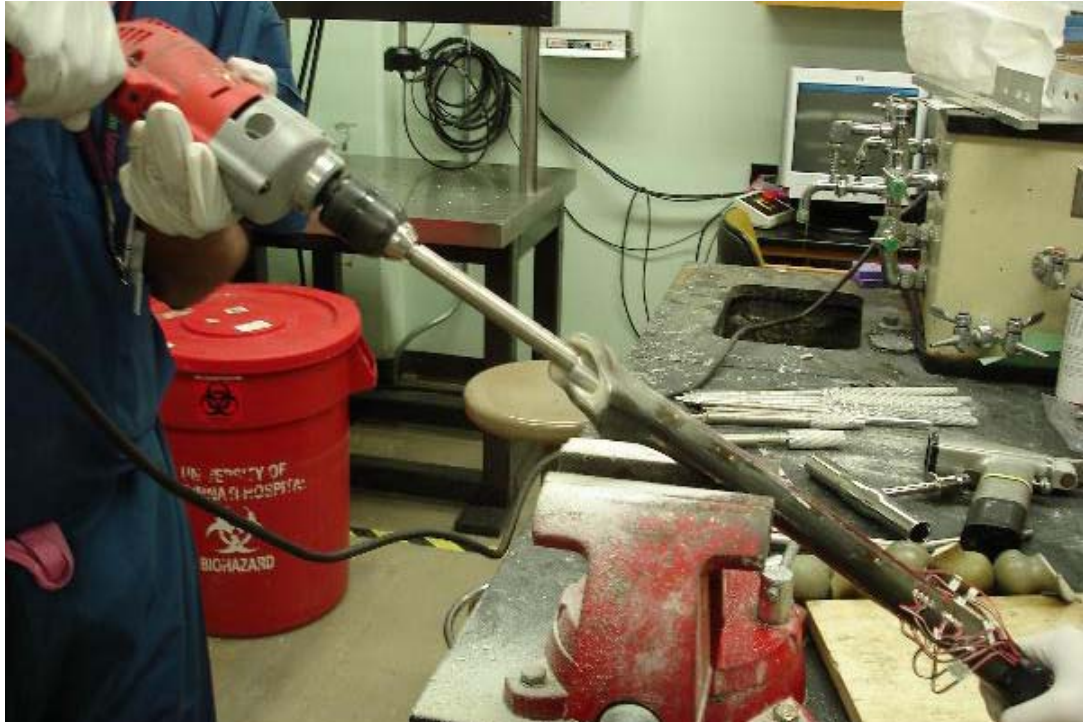
FIGURE 21. Orthopedic surgeon performing reaming process.
