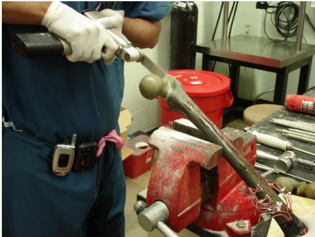
FIGURE 19. Removal of femoral head using Stryker power saw.
