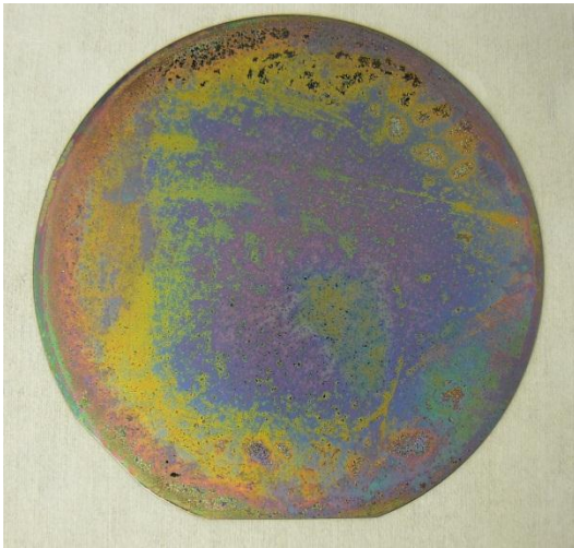
Figure 31: Ge device wafer following polyboron diffusion 850°C in RTP 5 minutes followed by oxidation and etching
