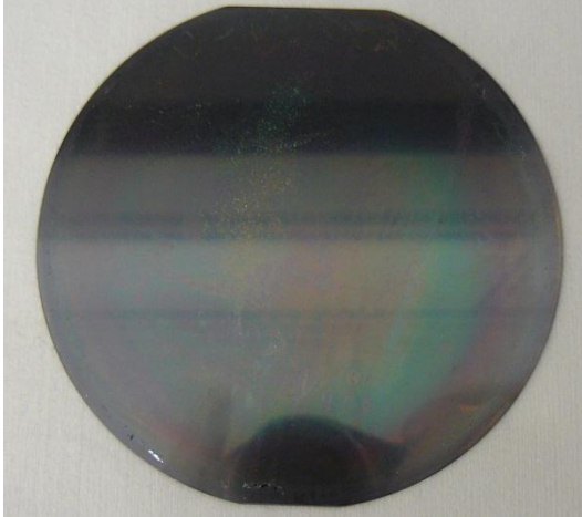
Figure 38: 10% SnGe after polyboron diffusion 850°C, wet oxidation, and etching to remove polyboron film
