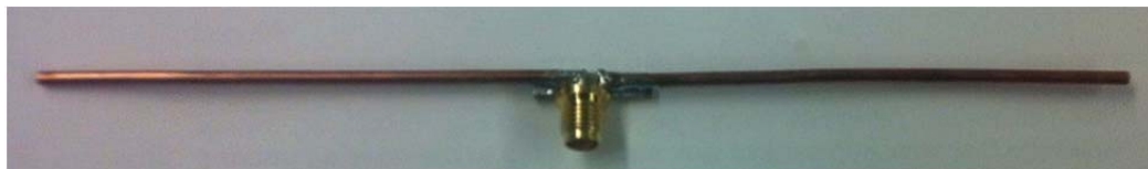
Figure 38. 915MHz half-wavelength wire dipole antenna.
