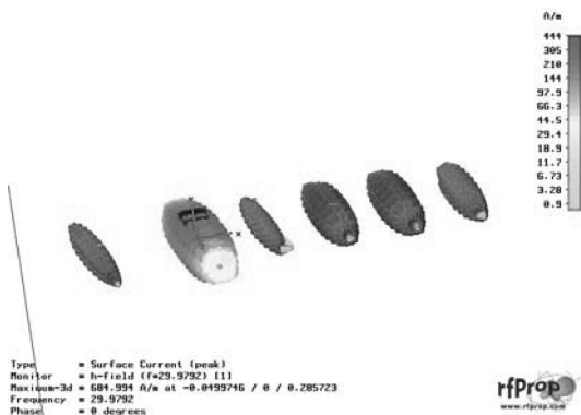
Fig. 1a Yagi-Uda antenna – surface current. in time domain (animation)
