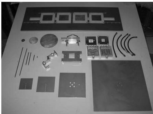
Fig. 6.a Patch array antenna – top view and all setup
