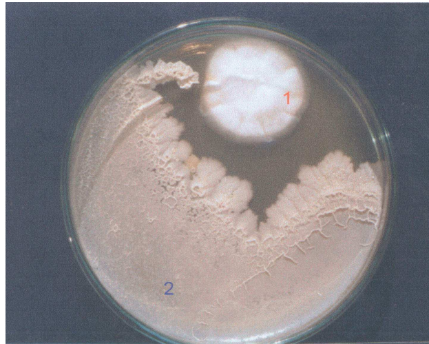
Figure 1: A colony of yeasts and moulds of the isolated infected emulsion on nutrient agar in Petri's vessel
