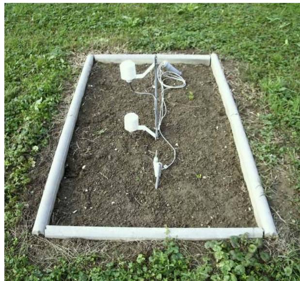
Figure 1. Equipment for temperature measurements at 5 cm and 50 cm above ground.
