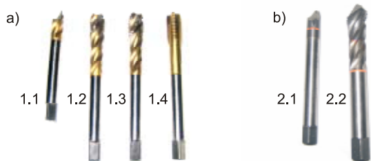
Figure 5. The appearance of damaged cutters prior to thread cutting in the sleeve: a) thread cutters with protective coating TiN; b) thread cutters with TiC protective coating
