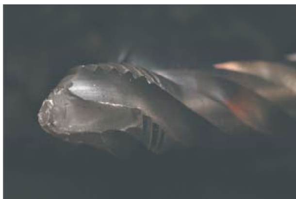
Figure 6. Appearance of the cracked surfaces of the thread cutter (macro record)
