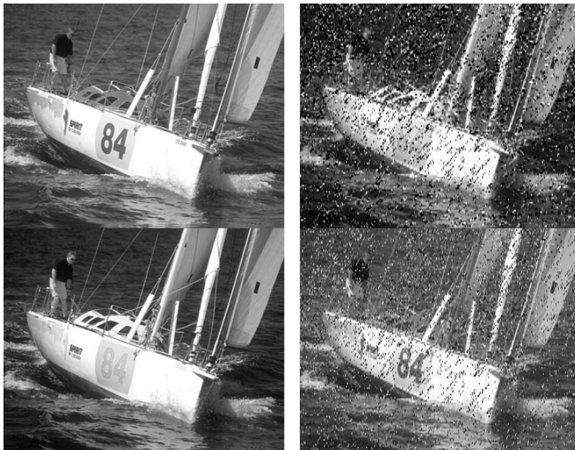
Fig. 4 Subjective check of transmission quality – comparison of input RGB and B&W images with transmitted images that are overlaid by the transmission errors (only example without specification)
