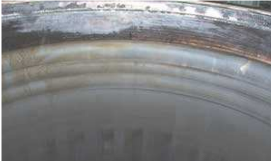
Figure 2b: Surface of cylinder bore after honing
