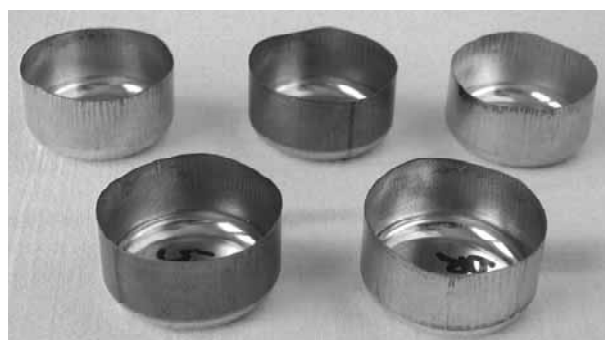
Figure 2. Drawn cups of tinplate for determining the ear height
