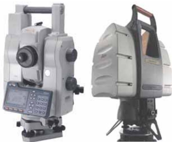
Fig. 1. Robotized total station and laser scanner
