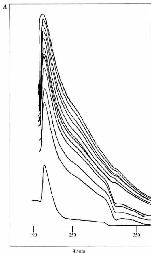
Figure 1. Alkaline cleavage of organic materials from Swanton sandy loam. 0.5 g of soil suspended in 25 mL of phosphate buffer, pH = 10.5. Reaction quenched by adjusting the pH to 8.0 and spectra recorded after filtering. Time of quenching from bottom curve up: 0; 1.0; 1.23; 2.13; 3.18; 4.19; 5.17; 9.50; 14.0; 19.95 and 23.0 min.
