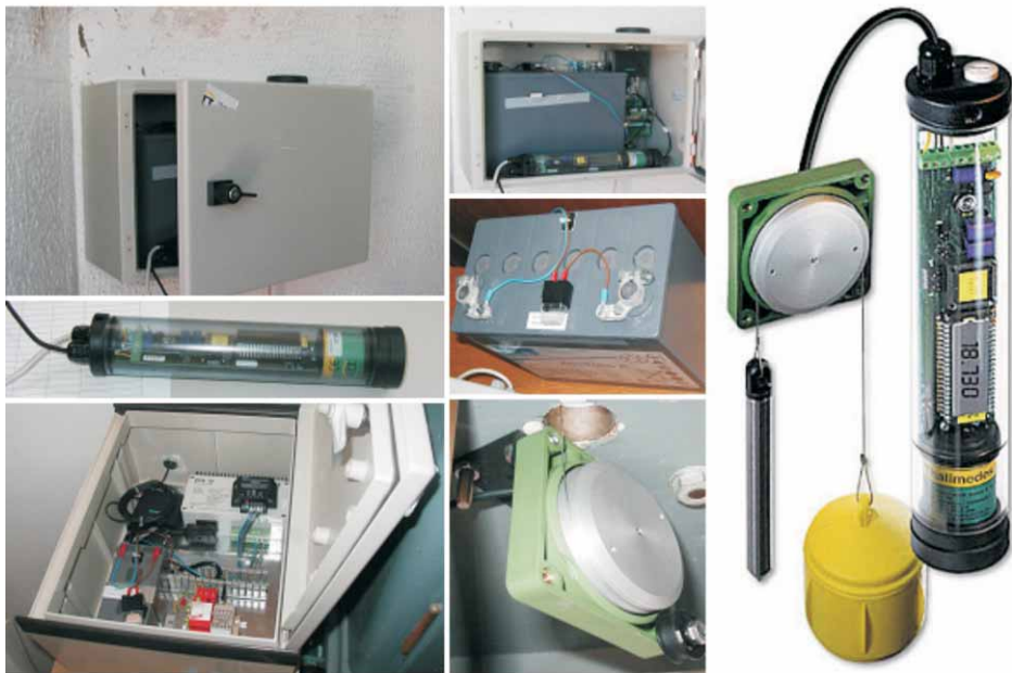
Figure 11. OTT Thalimedes instrument with additional equipment before and after the installation.
