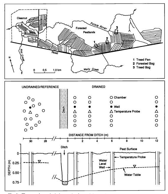
Fig. 1. The experimental design at the forested bog. The setup was exactly the same at the other two locations with the exception of that  $CH_4$  storage measurements and peat cores were only taken from the forest bog.
