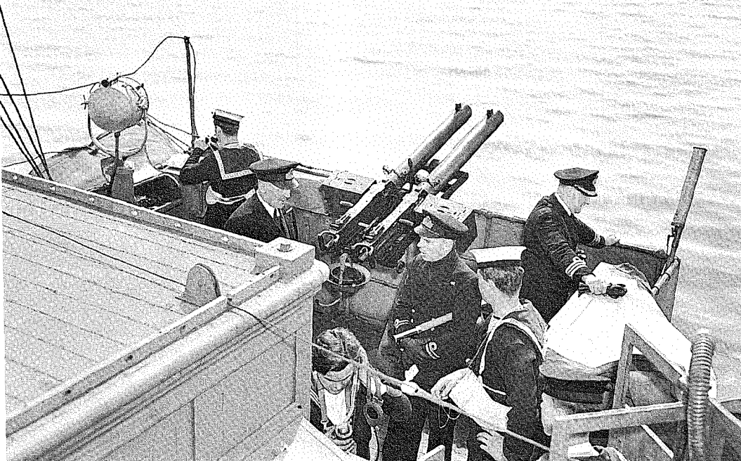
The original corvette bridge, like HMCS Moncton's seen here, during work-ups in May 1942, was ill-suited to the demands of war. The charthouse, in the left foreground, housed the ship's only compass — a magnetic one — and the trace recorder for the primitive type 123A asdic set, but the captain had to fight his ship from outside and the charthouse itself prevented a full 360 degree view of events. The cramped bridge wings did well to accommodate the twin .50 calibre machine guns seen here.
