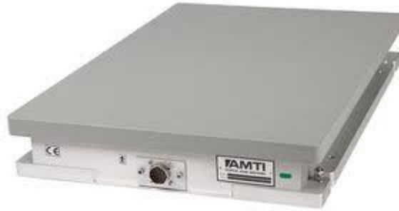
Figure 6: AMTI force plate used in the experiment
