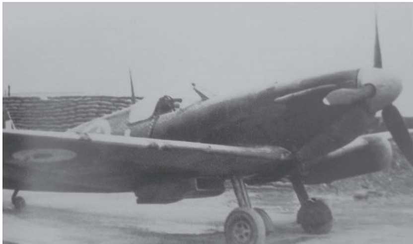
A Spitfire MkIIa with a 40 gallon single port wing fixed fuel tank. [ http://s412.photobucket.com/user/ruspren/media/ruspreno01/IMG_0703_zpsa8bob786.jpg.html ]
