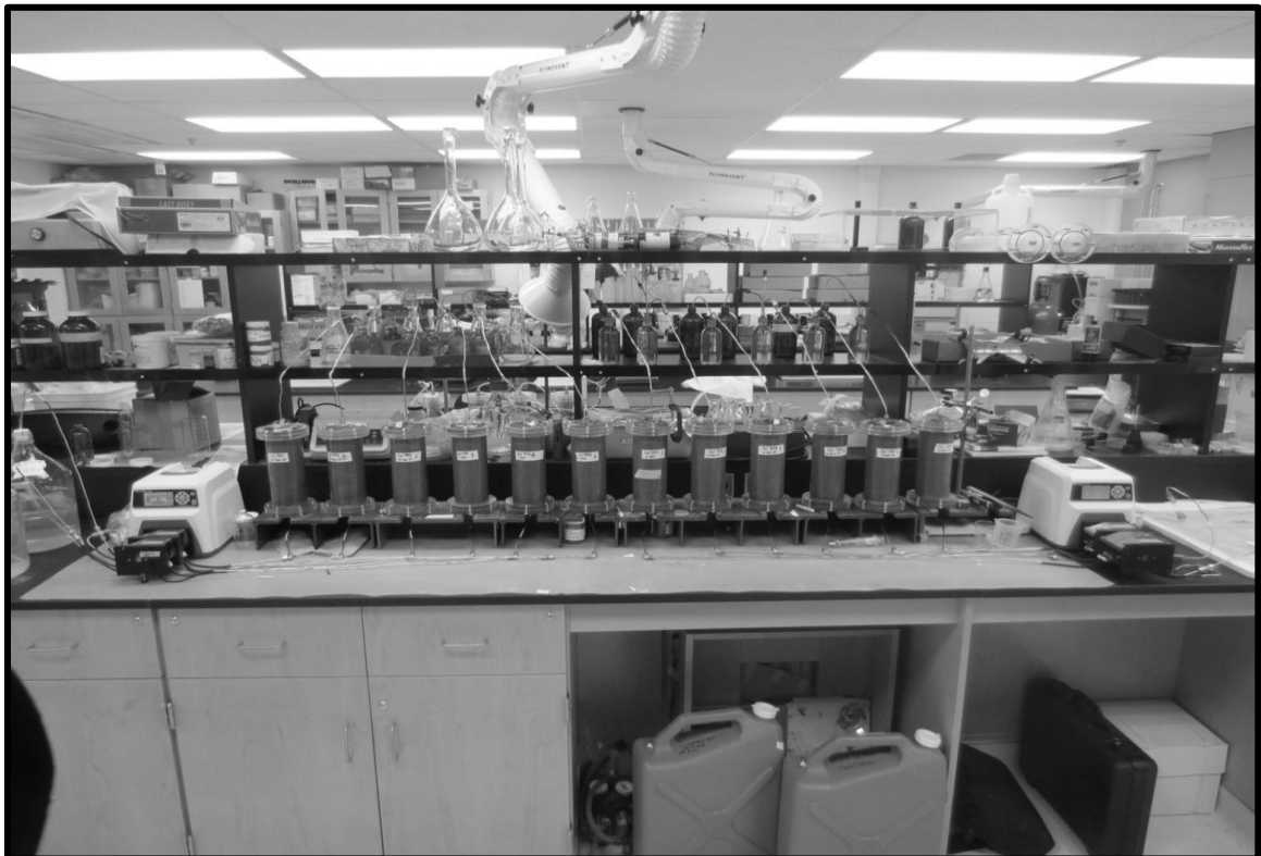
Figure A1: An illustration of the bench-scale set-up following bioreactor packing and attachment to GW reservoirs.
