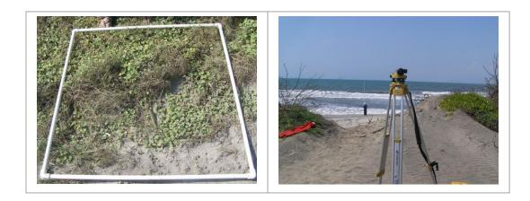
Figure 13. 1 m<sup>2</sup> quadrat to identify and quantify vegetation (left) and topographic profile along dunes, the latter using an AT G6 Topcon level (right).
