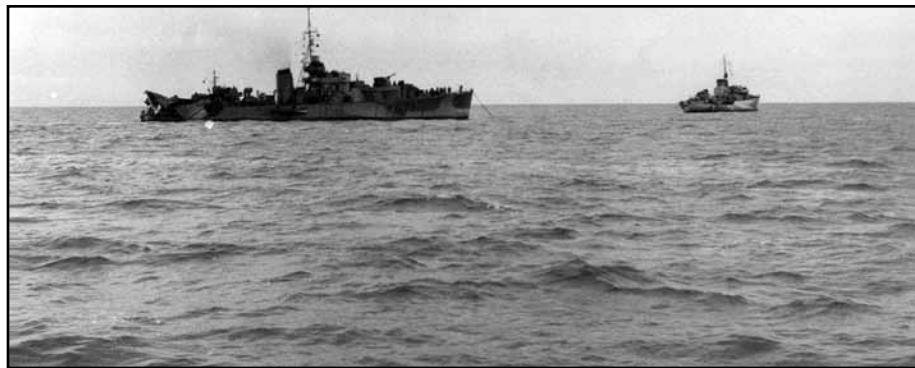
HMCS Magog under tow after the frigate was hit by a torpedo from U-1223 on 14 October 1944. The explosion demolished the 20-metre-long after section of the hull. Note the buckled remnants of the upper deck of the stern part of the ship, folded over top of the surviving superstructure.
