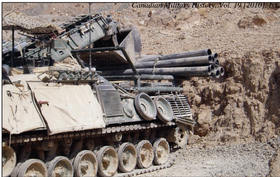
Badger Armoured Engineering Vehicles carried improvised fascines that were deployed via the bucket boom during the operation.
