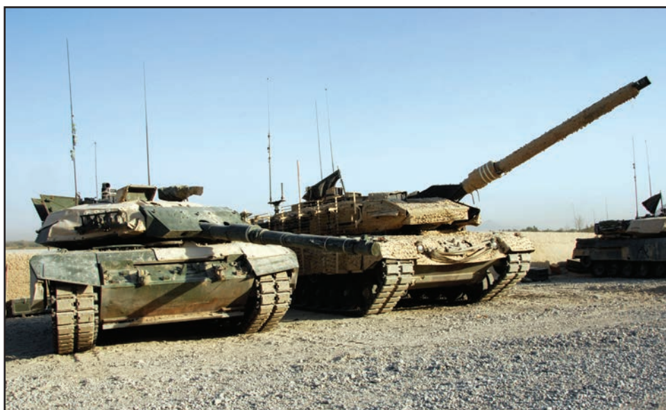
A Canadian Forces Leopard 1C2 Main Battle Tank (left) sits side-by-side with its newly-acquired cousin, the Leopard 2A6M.
