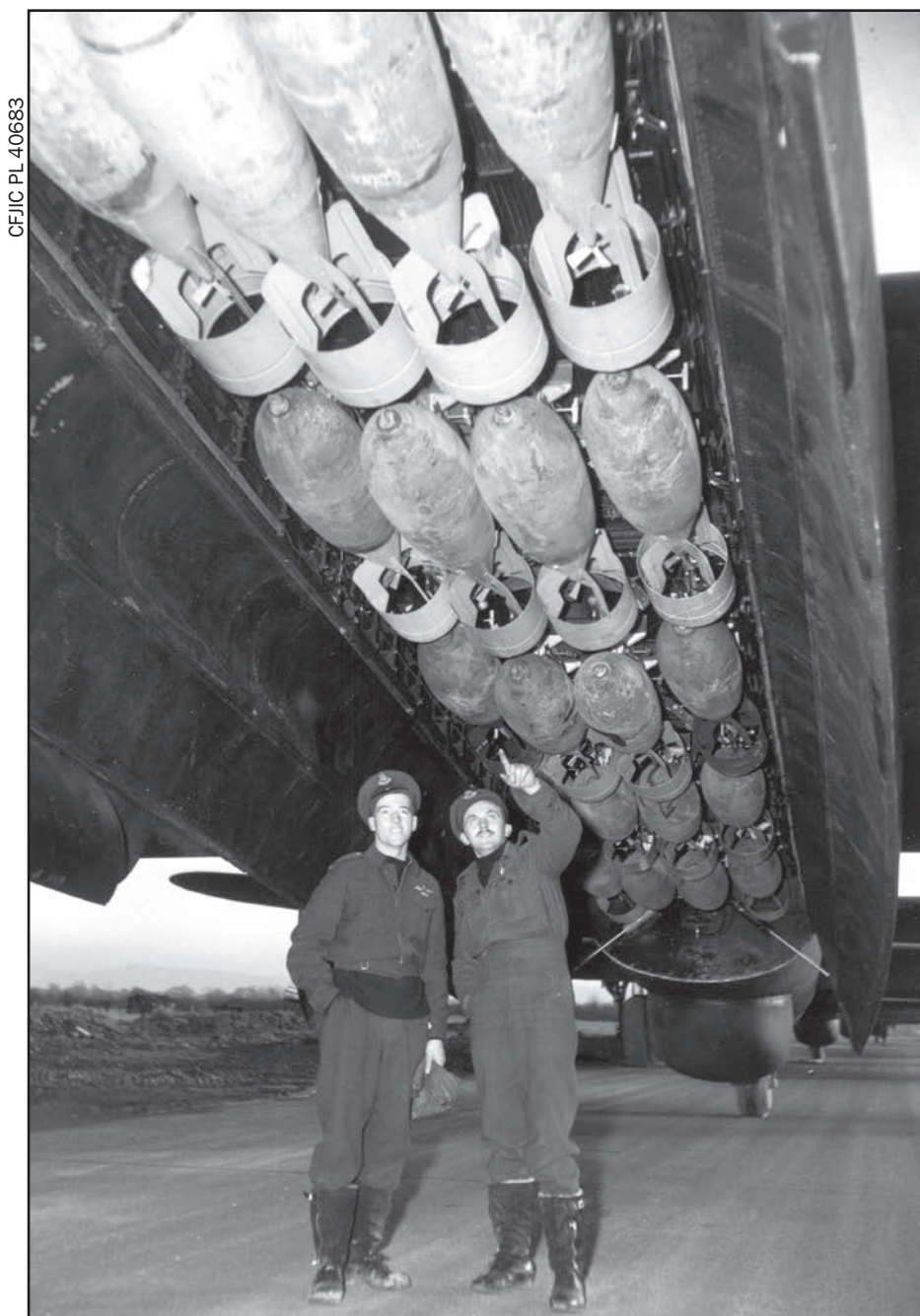
The pilot and bomb-aimer of a 428 Squadron Lancaster stand beneath the open bomb bay of their aircraft prior to an attack on an oil refinery in the Ruhr in late 1944. The short range to the target allowed a full load to be carried, in this case 500-pound, high explosive, general purpose bombs.
