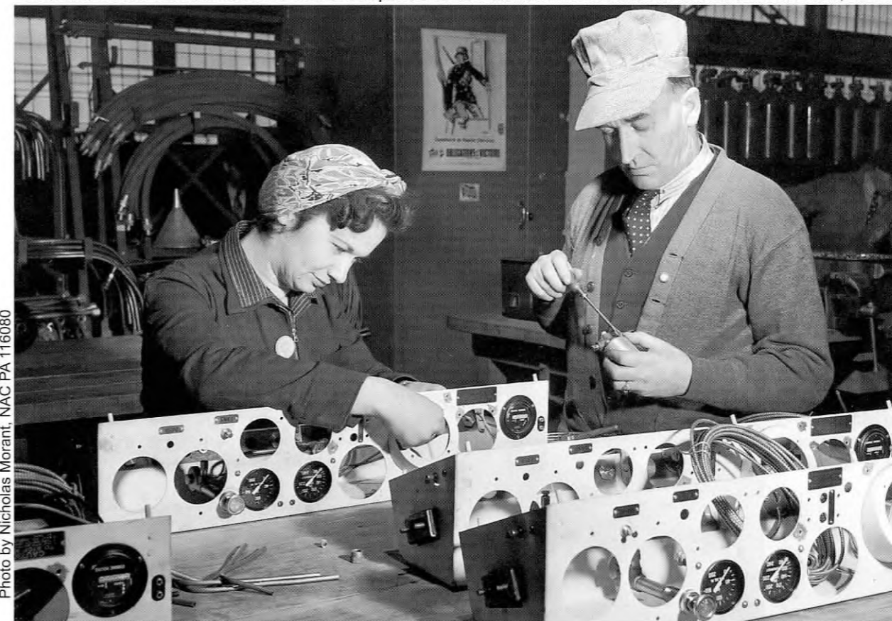
Male and female workers assemble instrument panels for Ram tanks at the Montreal Locomotive Works Plant, 1942.
