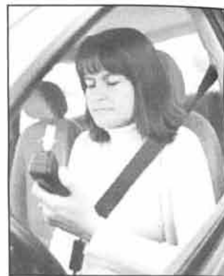
The ignition interlock system is one whereby the car won't start if the driver's blood-alcohol is too high.
