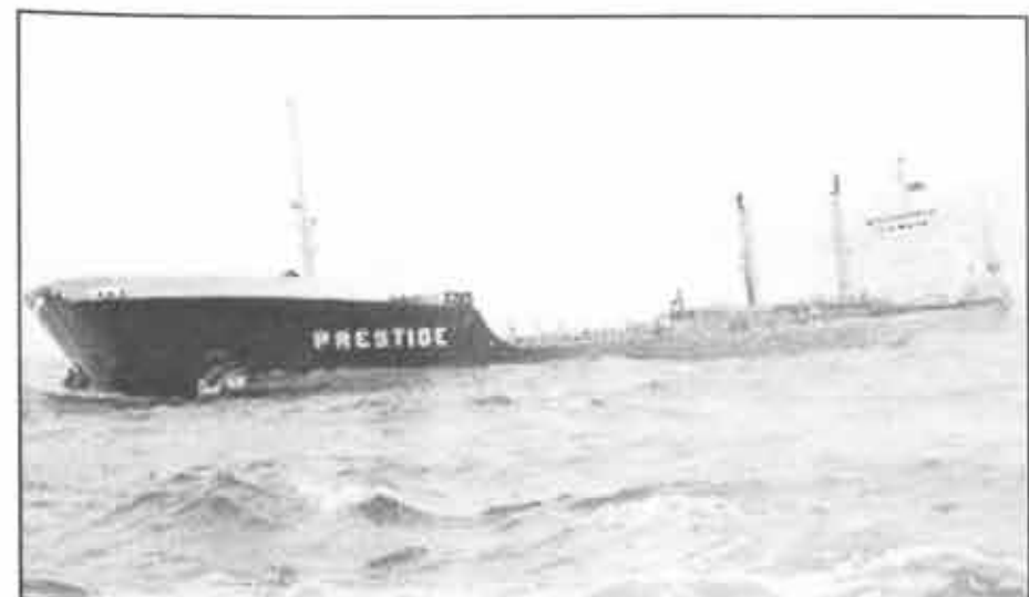
The Prestige's single hull developed cracks in a storm on November 13 before eventually splitting in two and sinking on November 19.
