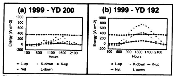
Figure 5.5 - Diurnal radiation balance for met site on (a) cloudy and (b) cloudless day.
