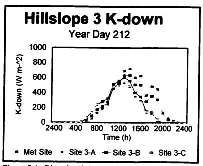
**Figure 5.4** - Diurnal variation of direct-beam solar radiation upon Hillslope #3 on YD 212.
