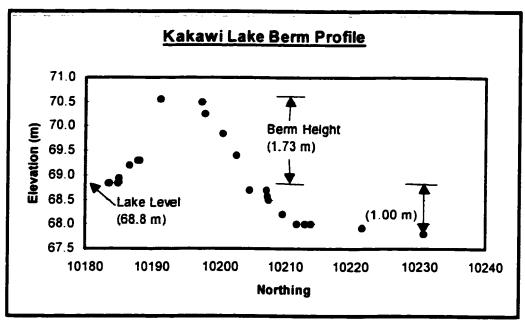
Figure 8.5 - Kakawi Lake discharge berm elevation profile.
