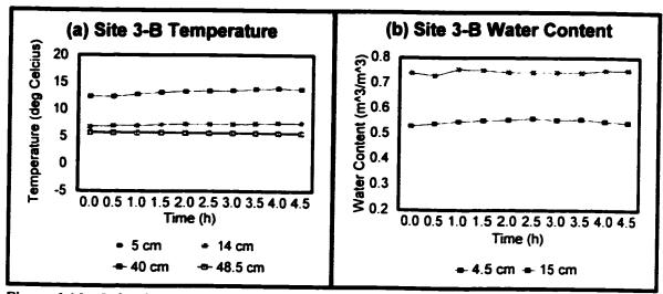
Figure 6.10 - Irrigation experiment Site 3-B changes in (a) soil temperature and (b) soil water content.
