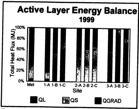
**Figure 6.16** - Active layer heat balance components expressed as percentage of total  $Q_G$  for the 1999 study period.  $Q_L$  for sites on hillslope 2 is not included.
