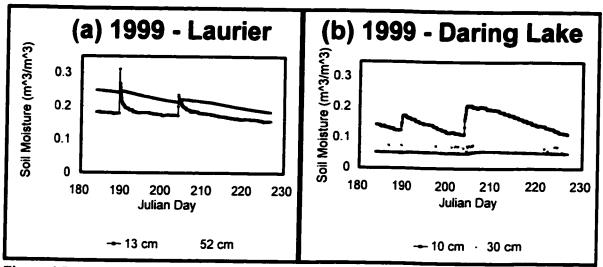
Figure 6.7 - Daily soil moisture contents measured at depth at (a) Laurier met site (hillslope) and (b) Daring Lake met site (relatively flat ground) during 1999 field season.
