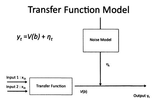
Figure 6 Schematic representation of a transfer function model with multiple inputs (Helfenstein, 1996)
