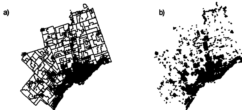
Figure 4.2.2: A comparison of a) regular enumeration units with b) dasymetric (residential land only) enumeration units
